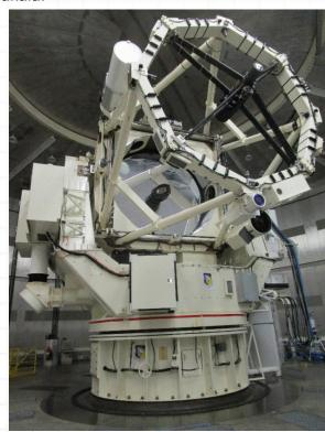
The 3.6-meter, 75-ton Advanced Electro-Optical System (AEOS) telescope shown above is the largest optical telescope in the Department of Defense. In addition the Maui Space Surveillance System facility houses several other telescopes ranging from 0.4 to 1.6-meters. Photo credit: AFRL
